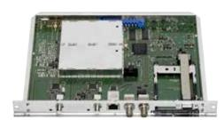
Converts two digital HDTV satellite signals (DVB-S2) to two Multicast modulated data streams. ASI input and an ASI output (ASI = Asynchronous Serial Interface acc. EN 50083-9) as well as a 100 MBit LAN interface (Ethernet).
