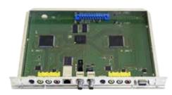
Converts two analogue video and audio signals into two MPEG2 data streams. These data streams are outputted at the ASI interface or LAN (IPTV) interface.
