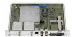
Cassette has ASI input and ASI output (ASI = Asynchronous Serial Interface acc. EN 50083-9) as well as a 100 MBit LAN interface (Ethernet).
