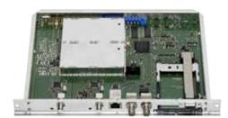
Converts two digital HDTV satellite signals (DVB-S2) to 16 x SPTS in Unicast or Multicast modulated data streams. ASI input and an ASI output (ASI = Asynchronous Serial Interface acc. EN 50083-9) as well as a 100 MBit LAN interface (Ethernet).
