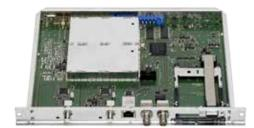
This cassette processes up to 8 transport streams delivered via IP (SPTS) or ASI and converts into 2 freely selectable COFDM channels. Interfaces include ASI input and ASI output (ASI = Asynchronous Serial Interface acc. EN 50083-9) as well as a 100 MBit LAN interface (Ethernet).
