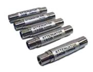
BL type attenuators have a frequency range from 100KHz ~ 860MHz and have an input/output impedance of 75ohm. They are available in 3dB, 6dB, 12dB, 18dB and 24dB attenuation levels.
